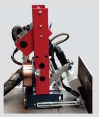
Also available with flue gas extraction nozzle to be connected to any supplied flue gas extraction system
