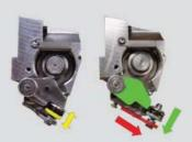
In-house developed push-pull package with a hand-grip barely larger than that of a package without engine. A great deal of attention has been paid to the wire feed-throughput and the adjustment of the pressure on the counter-pressure wheel.
